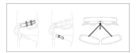
• Check the condition of the equipment loops (cuts, wear, tears...).
