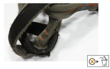
• Worn out belay loop and tie-in point
